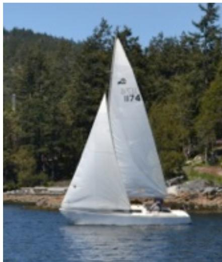
The accomplished naval architect Ben Seaborn took up the challenge, taking his design ideas to Ed Hoppen's Eddon Boat Works in Gig Harbor. He and his shipwrights came up with a method of home construction using bulkheads, long stringers and marine plywood sealed with fibreglass, the boat being built upside down. The plans could be bought cheaply (now from the Thunderbird International Class Association "ITCA"), and the boat can be built at home in under 2,000 hours (so they say...).
