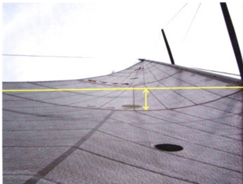
Picture #2 Mainsail trim. The slightly flatter shape has been induced using the Cunningham and increasing the outhaul. The traveller has also been dropped to position the boom in the centre or slightly to leeward, and the sheet has been trimmed to have the upper telltale almost stalling.
